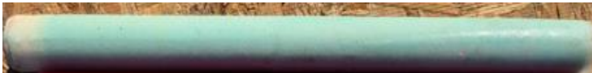
Fig. 2: Gel surfactant in a water-soluble shell.
