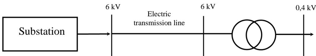
**Figure 1. Schematic diagram of the 6 kV rural power supply system**
