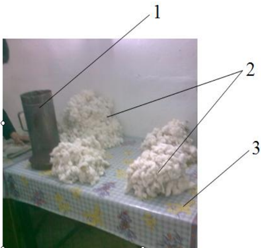
Figure 2. Sampling process in the laboratory room to determine the fine contaminants in the raw cotton.
