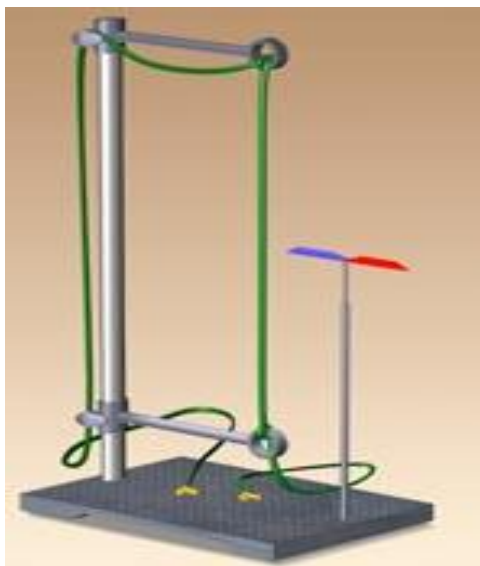
Figure 1. Oersted's experiments on the formation of a magnetic field around a constant current.
